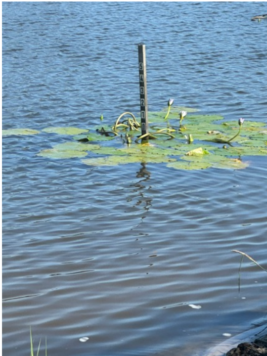
Water depth marker installed in Northern dredge pond.
